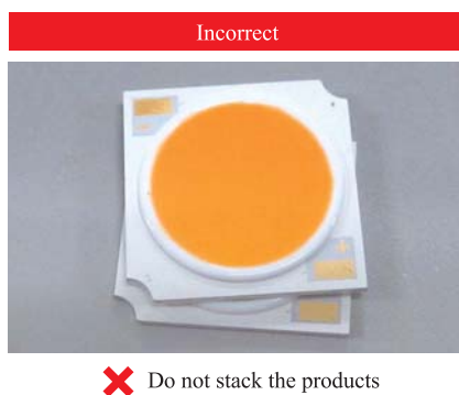
■Figure 9 Incorrect stacking of LED packages
